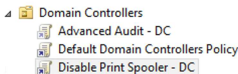
Figure 10 "Disable Print Spooler – DC" GPO Applied to Domain Controllers
